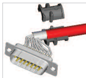
Attach the strain relief around the cable
