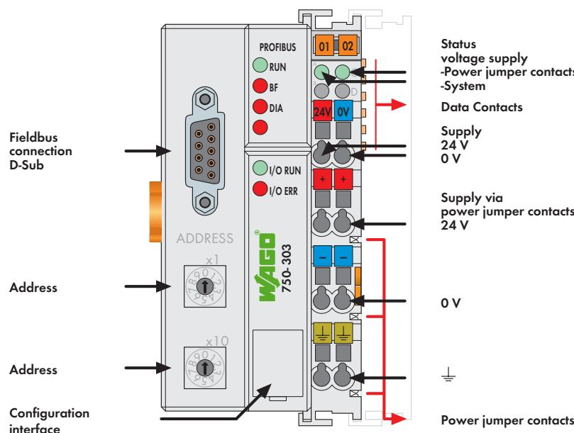
This buscoupler connects the WAGO-I/O-SYSTEM as a slave to the PROFIBUS fieldbus.
