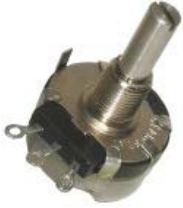
53 Series Industrial Potentiometer, Conductive Plastic Element, Solder lug Terminals, 2 W Power Rating, 5 kOhm Resistance Value
