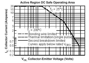
www.element14.com www.farnell.com www.newark.com There are two limitations on the power handling ability of a transistor: average junction temperature and second breakdown. Safe operating area curves indicate  $I_C - V_{CE}$  limits of the transistor that must be observed for reliable operation; i.e., the transistor must not be subjected to greater dissipation than the curves indicate.
