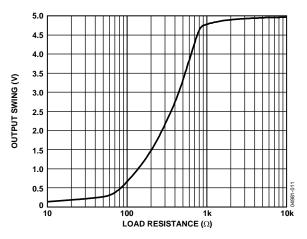
Figure 11. Output Swing vs. Load Resistance
