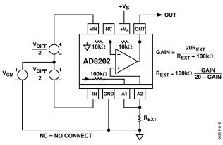
Figure 43. Adjusting for Gains Less than 20
