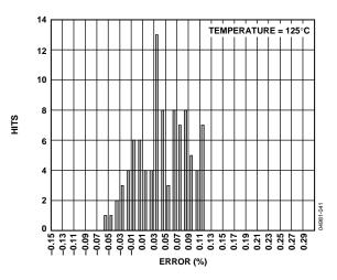
Figure 23. MSOP Gain Accuracy, Temperature = 125°C
