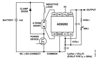
Figure 50. 2-Pole Low-Pass Filter
