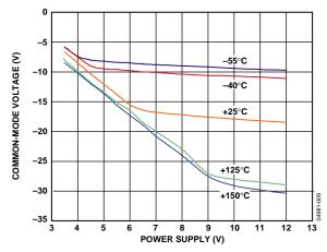
Figure 9. Negative Common-Mode Voltage vs. Voltage Supply
