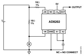
Figure 42. 4 to 20 mA Current Loop Receiver
