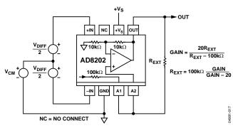
Figure 44. Adjusting for Gains > 20
