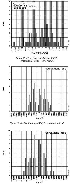
Figure 20. Vos Distribution, MSOP, Temperature = 125°C
