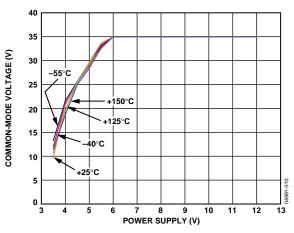
Figure 10. Positive Common-Mode Voltage vs. Voltage Supply
