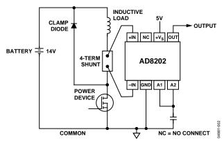
Figure 2. High Line Current Sensor
