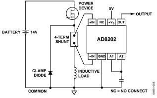
Figure 3. Low Line Current Sensor
