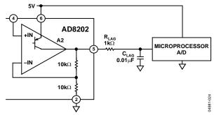
Figure 51. Recommended Circuit for Driving CMOS A/D
