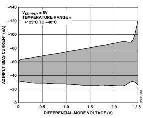
Figure 41. A2 Input Bias Current vs. Input Voltage and Temperature. The Shaded Area is the Bias Current from  $+125^{\circ}$ C to  $-40^{\circ}$ C.
