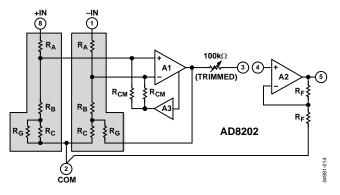
Figure 40. Simplified Schematic
