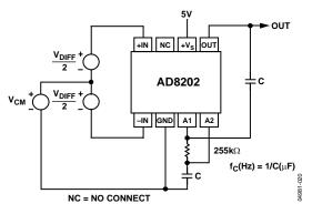
Figure 47. 2-Pole, Low-Pass Filter
