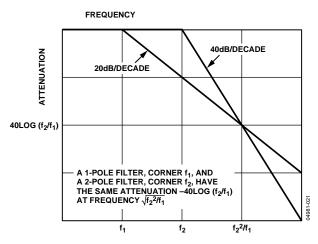
*Figure 48. Comparative Responses of 1-Pole and 2-Pole Low-Pass Filters*
