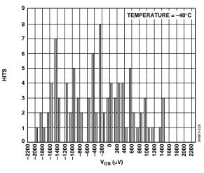
Figure 21. V<sub>os</sub> Distribution, MSOP, Temperature =  $-40^{\circ}$ C
