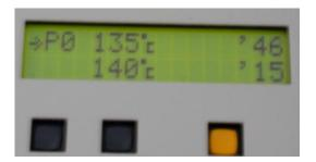
An arrow points the field, to modify it, press **C**, a star replaces the arrow, modify the value thanks to **A** button to decrease or **C** button to increase.
