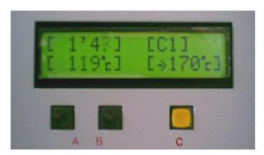
On the top: time and cycle phase (C1 preheating, C2 reflow and C3 cooling).
