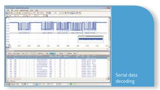
The PicoScope 6000 Series oscilloscopes are well-suited to serial decoding, with a deep memory buffer that allows them to collect long, uninterrupted sequences of data. This allows the capture of thousands of frames or packets of data over several seconds. The scopes can decode up to four buses simultaneously with independent protocol selection for each input channel.
