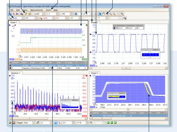
Movable axes: The vertical axes can be dragged up and down. This feature is particularly useful when one waveform is obscuring another. There's also an Auto Arrange Axes command. Automatic measurements: Display calculated measurements for troubleshooting and analysis. You can add as many measurements as you need on each view. Each measurement includes statistical parameters showing its variability.
