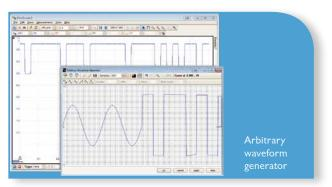
Generate standard waveforms from DC to 20 MHz (all models) or define your own using the power of the built-in 12-bit, 200 MS/s arbitrary waveform generator (B models only). You can import arbitrary waveforms from data files or draw them using the built-in AWG editor.
