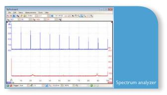
With the click of a button, you can open a new window to display a spectrum plot of selected channels. The spectrum analyzer allows signals up to 500 MHz (depending on the scope model) to be viewed in the frequency domain. A full range of settings give you control over the number of spectrum bands, window types and display modes.
