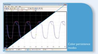
See old and new data superimposed, with new data in a brighter color or shade. This makes it easy to see glitches and dropouts and to estimate their relative frequency. Choose between analog persistence and digital color, or create a custom display mode.
