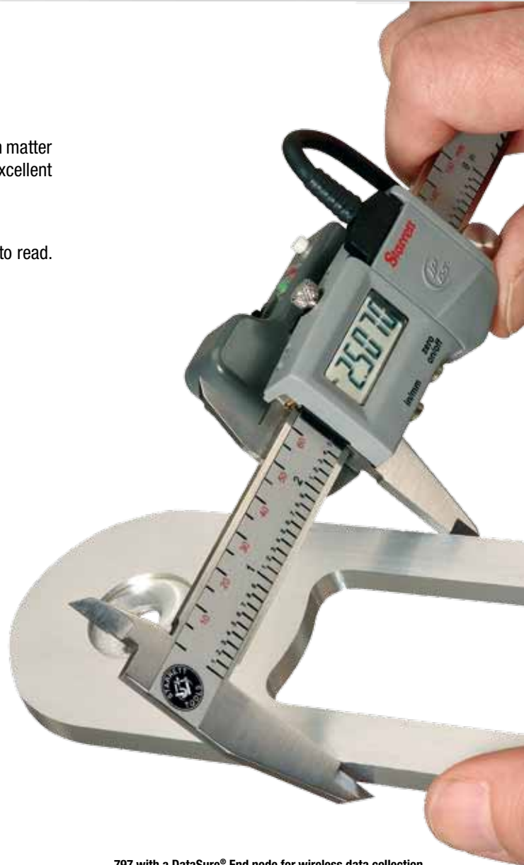
797 with a DataSure® End node for wireless data collection.
