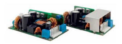
The new TOP-100 Series AC/DC Power Supplies feature the highest power rating in the industry standard  $2.0'' \times 4.0''$  (50.8 x 101.6 mm) footprint. They can supply up to 100 W output power with convection cooling over an industrial operating temperature range of  $-25^{\circ}$ C to  $+50^{\circ}$ C. This performance could be realized by a state of the art design providing an extremely high efficiency of >90 % which eliminates the need for a dedicated power supply cooling fan.
