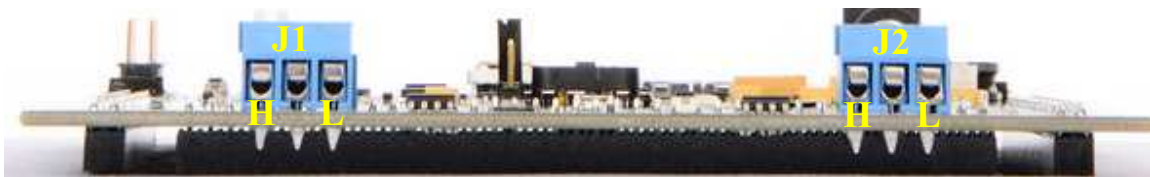
Figure 2-4. J1, J2 Screw Terminal Block for CAN Bus
