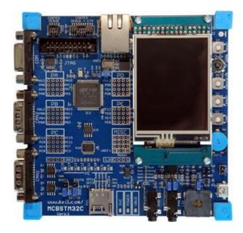
The Keil MCBSTM32C Evaluation Board enables you to create and test working programs based on the STMicroelectronics STM32 Connectivity Line family of ARM Cortex™-M3 processor-based devices.
