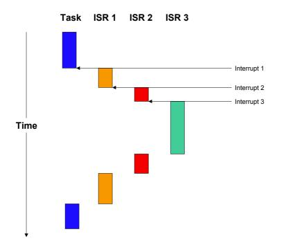
For applications requiring short interrupt latency, you may re-enable interrupts inside an ISR by using <code>OS\_EnterNestableInterrupt()</code> and <code>OS\_LeaveNestableInterrupt()</code> within the interrupt handler.
