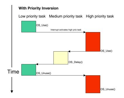
The low priority task claims the semaphore with OS\_Use(). An interrupt activates the high priority task, which also calls OS\_Use().
