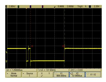
$t_{CD}$  is measured as 7250ns. The number of cycles calculates as follows: Cycles<sub>CD</sub> =  $t_{CD} / t_{Cycle}$ = 7250ns / 20.866ns = 347.46Cycles => 347Cycles
