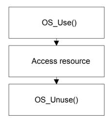
A resource semaphore contains a counter that keeps track of how many times the resource has been claimed by calling <code>OS\_Request()</code> or <code>OS\_Use()</code> by a particular task. It is released when that counter reaches 0, which means the <code>OS\_Unuse()</code> routine has to be called exactly the same number of times as <code>OS\_Use()</code> or <code>OS\_Request()</code>. If it is not, the resource remains blocked for other tasks.
