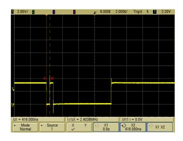
$t_{AB}$  is measured as 436.8ns. The number of cycles calculates as follows: Cycles<sub>AB</sub> =  $t_{AB} / t_{Cycle}$ =416.0ns / 20.866ns = 19.937Cycles => 20Cycles
