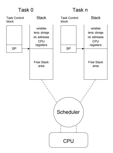
The scheduler deactivates the task to be suspended (Task 0) by saving the processor registers on its stack. It then activates the higher-priority task (Task n) by loading the stack pointer (SP) and the processor registers from the values stored on Task n's stack.
