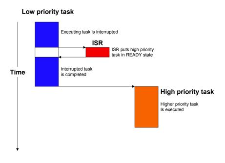
A pure cooperative multi-tasking system has the disadvantage of longer reaction times when high priority tasks become ready for execution. This makes their usage in embedded systems uncommon.
