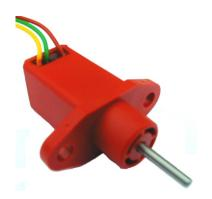
Conductive polymer potentiometer with 10mm linear effective travel for automotive and industrial applications. Connection via flying leads colour coded as detailed below, 200 mm in length. Standard spindle is 3mm diameter with a length of 29mm from fixing face., but other lengths area available upon request
