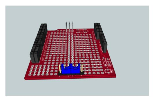
If you use the 6-pin male header jumpers to power the BUS, then you can only have +5V.
