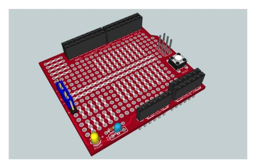
The kit includes the board and many extra components. What you finally end up installing on the ProtoShield will be based on your requirements. But in general, I recommend soldering all the female headers, as they are needed to bring all the signals and POWER from the chipKIT Uno32 board to the ProtoShield.
