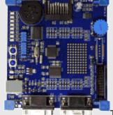
The Keil MCB2140 Evaluation Board introduces you to the NXP (founded by Philips) LPC2140 ARM family and allows you to create and test working programs for this advanced architecture.
