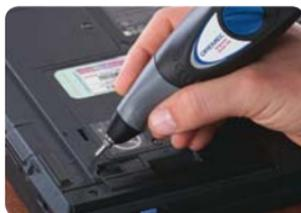
**Stroke adjustment dial.** Regulates engraving depth from fine lines to deep grooves.
