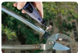
**FLAPWHEELS** Flapwheels grind and polish flat or contoured surfaces. They are used most effectively as a finishing sander after heavier surface sanding and material removal is completed.
