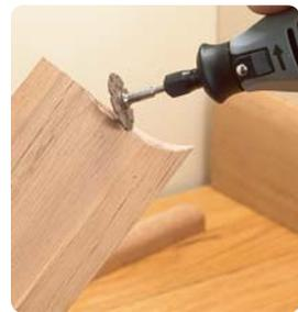
**CARBIDE CUTTING/SHAPING WHEEL - 543** For cutting and shaping on soft and hard woods, fiberglass, plastics and laminates. Do not use on metal. Mandrel included. Thickness .070" (1.8 mm).
