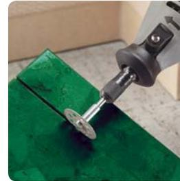
**DIAMOND WHEEL - 545** Great for cutting, sawing and carving of hard materials such as marble, concrete, brick, porcelain, ceramics, hard epoxy, soft and hard wood. Mandrel 402 is included. Thickness .023" (0,6 mm). Do not run in excess of 20,000 RPM.
