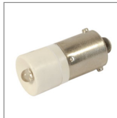
StarLED, BA9s LED-Lamp, 6V AC/DC, cold white
