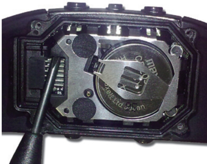
Figure 4-1. Removing Watch Module from Housing
