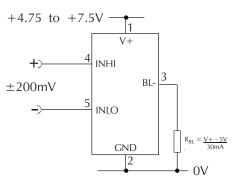
Measuring an input voltage referenced to a floating supply, i.e. the input voltage and the meter's power supply are isolated from each other. Ensure solder link LCOM is closed.
