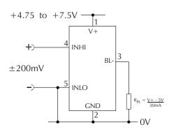
Measuring a single ended input voltage referenced to supply, i.e. the input voltage and the meter's power supply share the same 0V rail. Ensure solder link LCOM is open.
