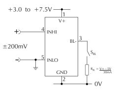
Measuring a single ended input voltage referenced to a split supply, i.e. the input voltage and the meter's power supply share the same 0V rail. Ensure solder link LCOM is open.
