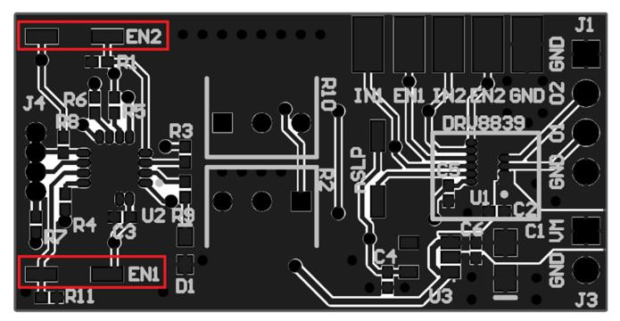
Figure 2. ENABLE Jumpers (EN1 and EN2)
