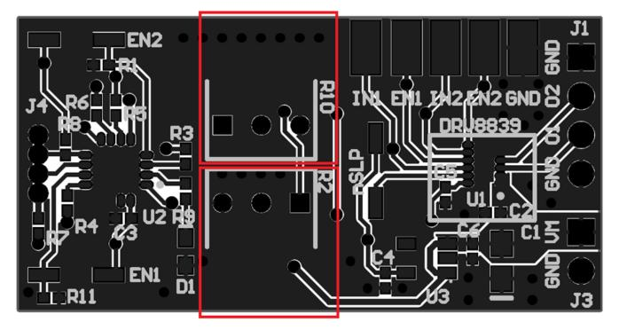
Figure 4. Speed Adjust Potentiometer (R2 and R10)
