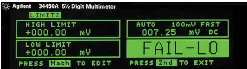
Figure 5. The display of 34450A in limit operation.
