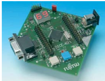
The MB90350, now with dual-operation flash.
