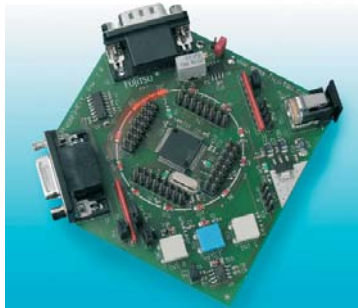
The MB91F267, offers three-phase motor control.
