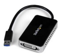
The USB32DVIEH USB 3.0 to DVI Adapter turns an available USB 3.0 port into a DVI output port with high resolution 1920x1200 video support. The adapter features a built-in 1-Port USB 3.0 hub, which offers a connection port in place of the USB port used for connecting the DVI adapter – an ideal workaround for Ultrabook™ or laptop users where only a limited number of USB ports are available.
