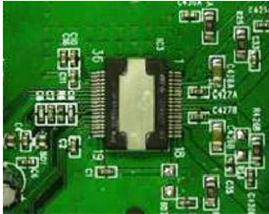
Sound Terminals™ are high performance, integrated single chips capable of digitally processing and amplifying audio signals maintaining a fully digital format from source to speaker, thus reducing the BOM, the design costs, the footprint area and at the same time improving the clarity of the sound.
