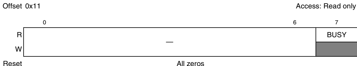
Figure 35. PIXIS VELA Status Register (PX_VSTAT)
