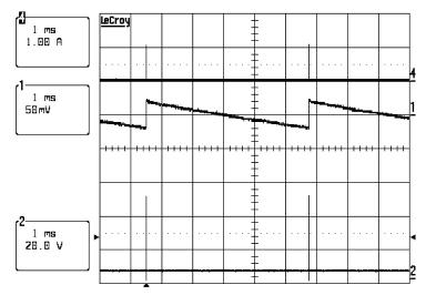
$$\label{eq:trace} \begin{split} & \text{Trace 4} = \text{Inductor Current} \\ & \text{Trace 1} = V_{\text{OUT}} \\ & \text{Trace 2} = \text{SW Node} \\ & V_{\text{IN}} = 48 \ \text{V}, \ \text{I}_{\text{OUT}} = 0 \end{split}$$
