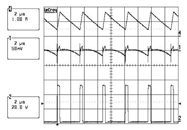
$\begin{array}{l} \mbox{Trace 4 = Inductor Current} \\ \mbox{Trace 1 = } V_{OUT} \\ \mbox{Trace 2 = SW Node} \\ \mbox{V}_{IN} = 48 \ \mbox{V}, \ \mbox{I}_{OUT} = 1 \ \mbox{Amp} \\ \mbox{Minimum Ripple Configuration (Option A)} \end{array}$
