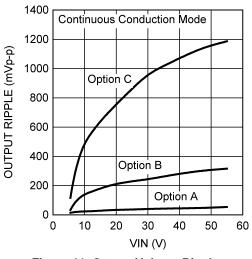
Figure 11. Output Voltage Ripple
