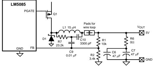
Figure 4. Minimum Ripple Using R7, C9, C10
