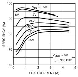
Figure 8. Efficiency vs Load Current
