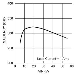
Figure 10. Switching Frequency vs. Input Voltage
