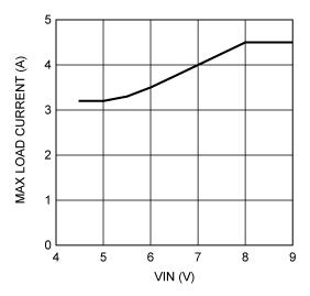
Figure 2. Maximum Load Current Derating
