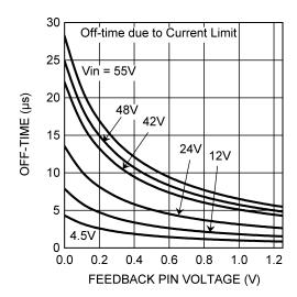
Figure 3. Current Limit Off-time vs. V<sub>IN</sub> and V<sub>FB</sub>
