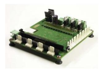
The BeBoPr Cape provides all the necessary I/O to control a Mendel/Reprap 3D-printer.
