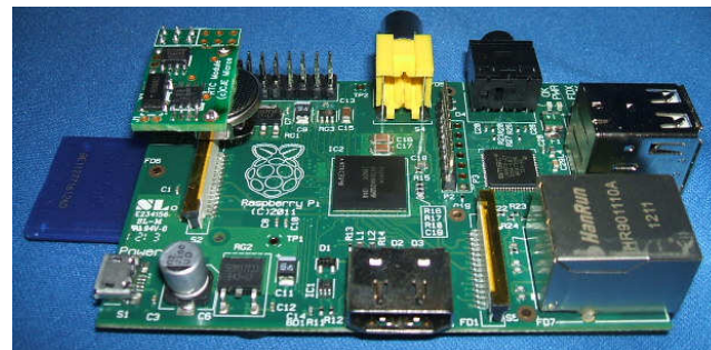
3. The RTC Module in place on the Raspberry Pi
