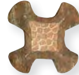
Indenter Crimp Cross-Section Across Axis
