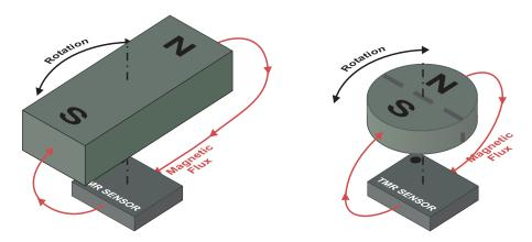
The sensor element free layers will align with the external field. As the applied field changes direction, the angle between the free layer and the pinned layer changes, changing the resistance of TMR elements, which changes the device output voltages.
