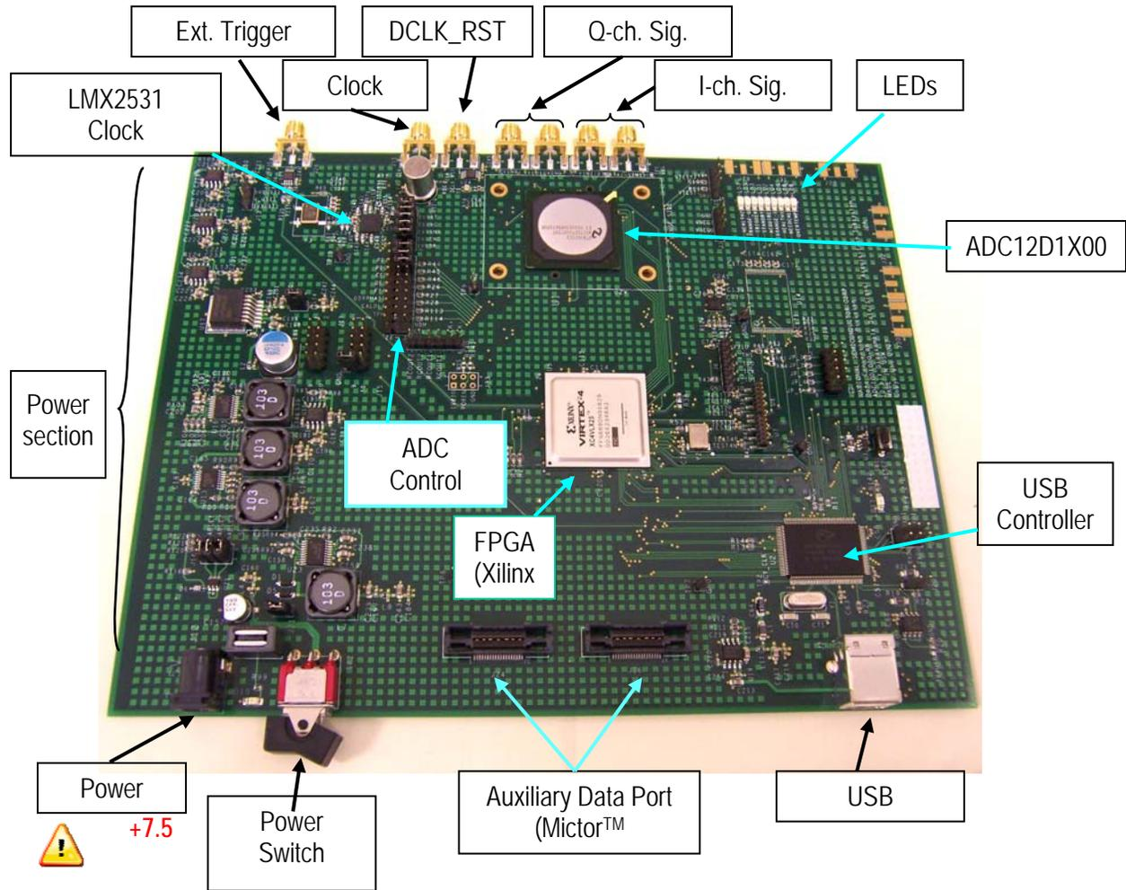
Figure 1: ADC12D1X00RB Board Layout
