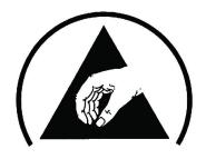
The ESD Protective Symbol identifies products designed to provide ESD control protection.
