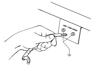
If you are not using a continuous or a constant monitor, a wrist strap should be tested while being worn at least daily. This quick check can determine that no break in the path-to-ground has occurred. Part of the path-to-groud is the perspiration layer on the person; an operator with dry skin may inhibit the removal of static charges and may cause a test failure.
