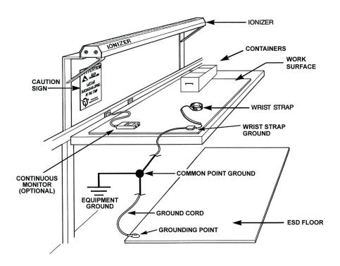
Per ESD Handbook ESD TR20.20-2008 section 2.4 "It should be understood that any object, item, material or person could be a source of static electricity in the work environment. Removal of unnecessary nonconductors, replacing nonconductive materials with dissipative or conductive materials and grounding all conductors are the principle methods of controlling static electricity in the workplace, regardless of the activity."
