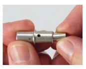
**Step 1:** Place crimp sleeve reducer into contact barrel.
