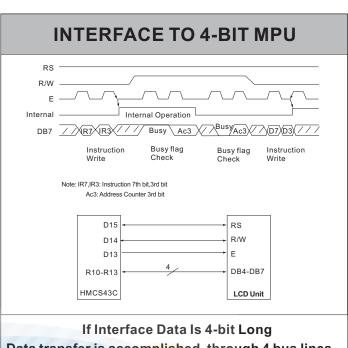
Data transfer is accomplished through 4 bus lines from DB4 to DB7. (while the rest of 4 bus lines from DB0 to DB3 are not used.)
