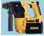
24V 2-mode SDS-Plus cordless hammer drill. Suitable for drilling anchors and fixing holes in concrete, brick and masonry from 4 to 22mm. Compact design and rear mounted battery for balance and comfort. Internal mechanism connected to external housings via spring dampeners resulting in lower vibration and reduced user fatigue. Impact energy 2.1J. Supplied with charger, 2 x 2.0Ah Ni Cd battery packs, grease tube and heavy duty carry case.
