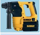
24V 3 mode SDS-Plus hammer drill. Internal mechanism connected to external housings via spring dampeners meaning significantly lower vibration. Supplied with charger, 2 x 2.0Ah Ni Cd battery packs, side handle, grease and carrying case.
