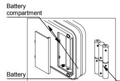
Remove the battery compartment cover and insert six batteries (LR6 AA size) into the battery compartment, taking extreme care that the polarities plus and minus is observed.
