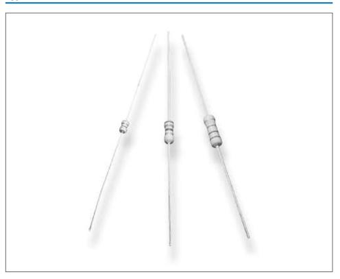
The resistive element comprises a thin film of carbon, deposited onto a high thermal conductivity ceramic core. Metal end caps are force fitted to the element prior to spiralling to value. Tinned copper lead wires are welded to the end caps and the components are then coated. One coat of phenolic resin is followed by three coats of epoxy resin. All resistors are tested for value and tolerance.
