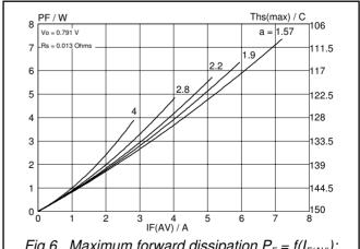
Fig.6. Maximum forward dissipation  $P_F = f(I_{F(AV)})$ ; sinusoidal current waveform where a = form factor  $= I_{F(RMS)} / I_{F(AV)}$ .
