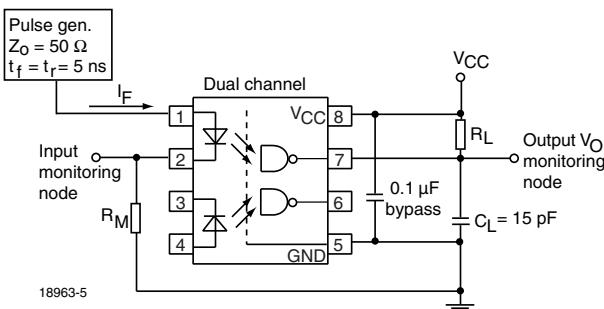
Fig. 2 - Dual Channel Test Circuit for  $t_{PLH}$ ,  $t_{PHL}$ ,  $t_r$  and  $t_f$
