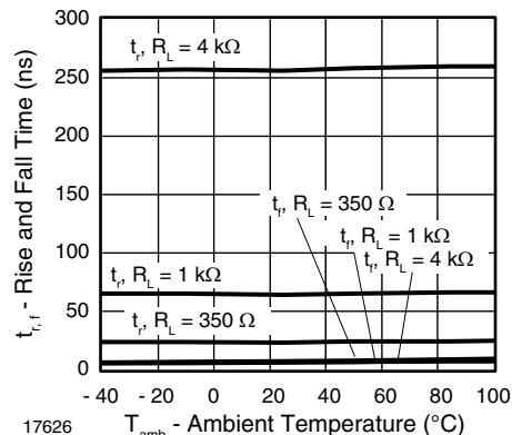
Fig. 21 - Rise and Fall Time vs. Ambient Temperature
