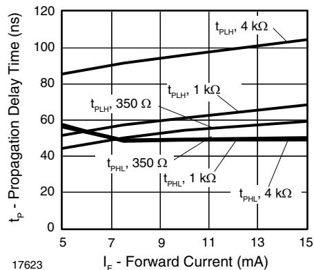
Fig. 18 - Propagation Delay vs. Forward Current
