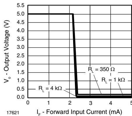
Fig. 16 - Output Voltage vs. Forward Input Current
