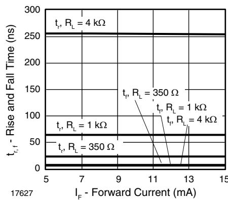
Fig. 22 - Rise and Fall Time vs. Forward Current
