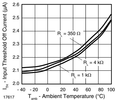
Fig. 12 - Input Threshold Off Current vs. Ambient Temperature
