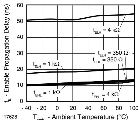
Fig. 23 - Enable Propagation Delay vs. Ambient Temperature
