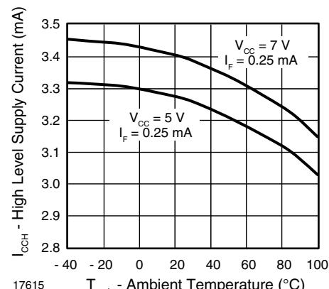
Fig. 10 - High Level Supply Current vs. Ambient Temperature
