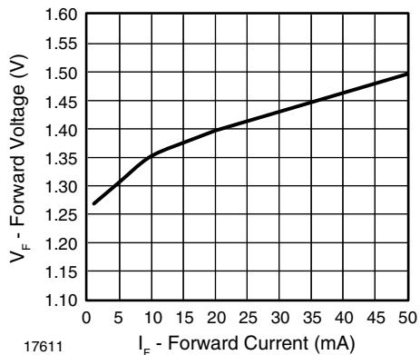
Fig. 7 - Forward Voltage vs. Forward Current
