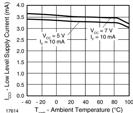
Fig. 9 - Low Level Supply Current vs. Ambient Temperature
