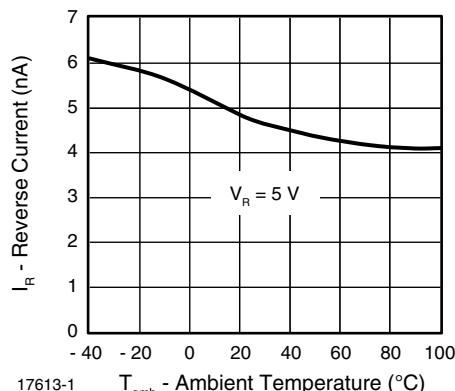
Fig. 8 - Reverse Current vs. Ambient Temperature
