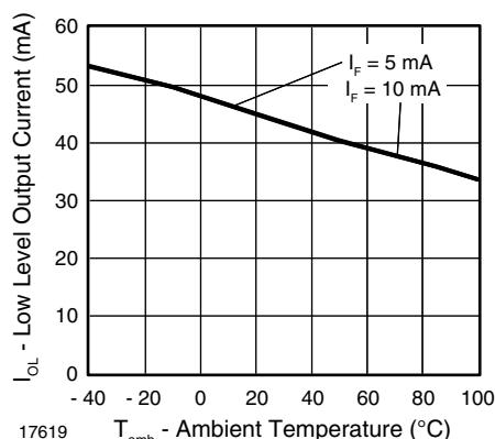
Fig. 14 - Low Level Output Current vs. Ambient Temperature
