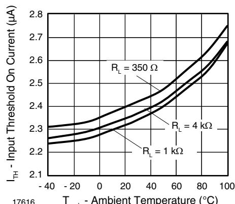
Fig. 11 - Input Threshold On Current vs. Ambient Temperature
