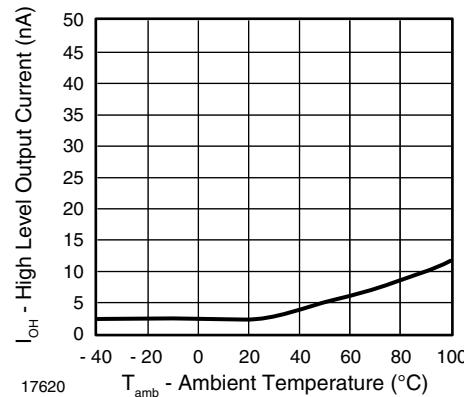
Fig. 15 - High Level Output Current vs. Ambient Temperature
