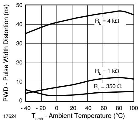
Fig. 19 - Pulse Width Distortion vs. Ambient Temperature
