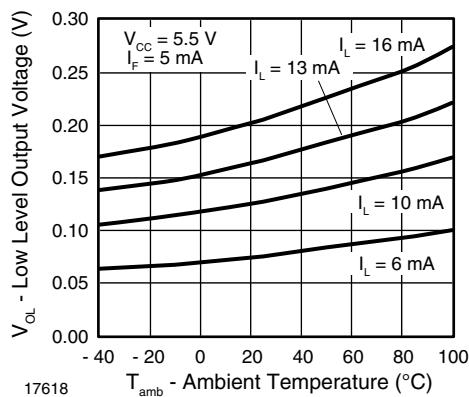
Fig. 13 - Low Level Output Voltage vs. Ambient Temperature
