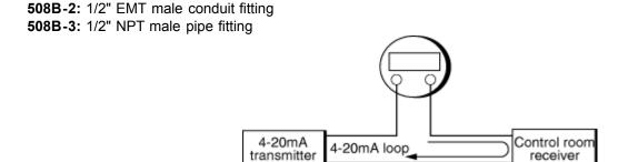
A Model **508B** process-loop indicator may be added to an existing 4-20 mA or 10-50 mA installation. No additional wiring is required, since the meter is powered directly by the current loop.
