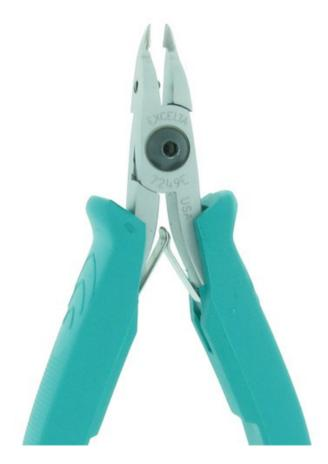
This tool is made of extruded 1% carbon tool steel. The cutting blades are induction hardened to RHC 63-65. Long soft cushioned ergonomic handles are designed for comfort and are ESD safe. Stainless steel leaf springs round out the package for positive and reliable action
