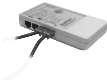
AX-110BT Realtime 10/100 Base-TX Ethernet Network Test Unit
