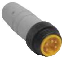
DeviceNet terminating resistor, 7/8" male connector, 5 poles.
