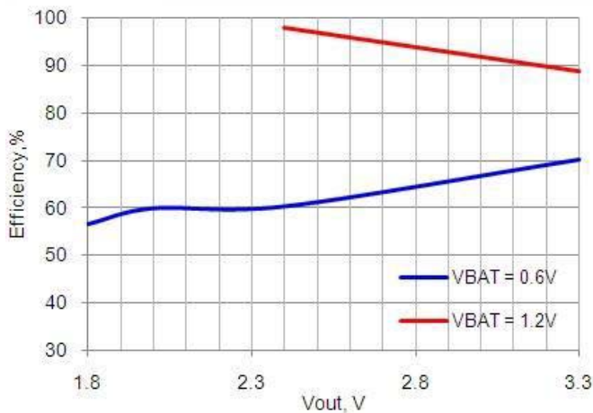
Figure 11-10. Efficiency vs V OUT I OUT = 30 mA, V BAT = 0.6 V and 1.2 V
