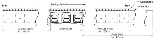
Packaging is referred to the international standard IEC 60286 -3:2007 rojection - 180° Vürth Elektronik eiSos GmbH & Co. KG MC & Inductive Solutions Max-Eyth-Str. 1
