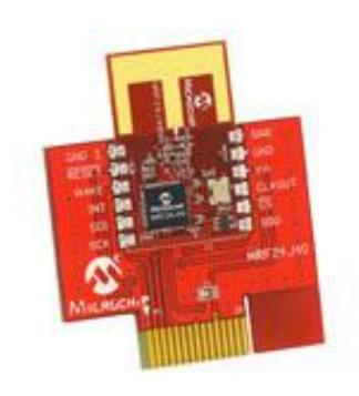
The MRF24J40MA PICtail Plus 2.4GHz Radio Frequency Card is built with the NEW agency-certified MRF24J40MA IEEE 802.15.4 RF transceiver module. The module is attached to a PICTail Plus carrier board allowing the RF Board to be used with an Explorer 16 development kit. Targeted for ZigBee, MiWi, and MiWi P2P wireless protocol applications, the MRF24J40MA is a perfect solution for low-cost, low-power complete embedded wireless PAN applications.
