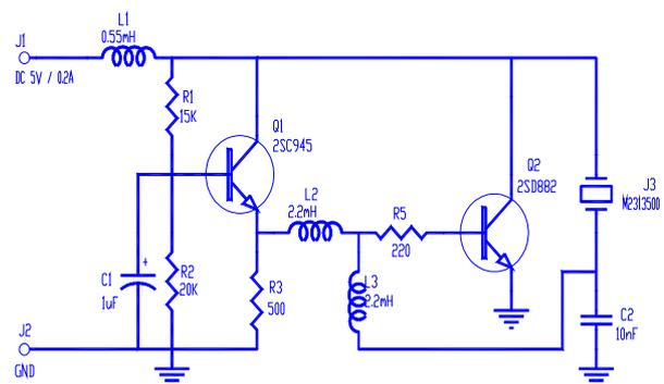
Remark: The negative side faces to the opening, the positive side faces to the liquid source, if driving circuit uses NPN transistor.
