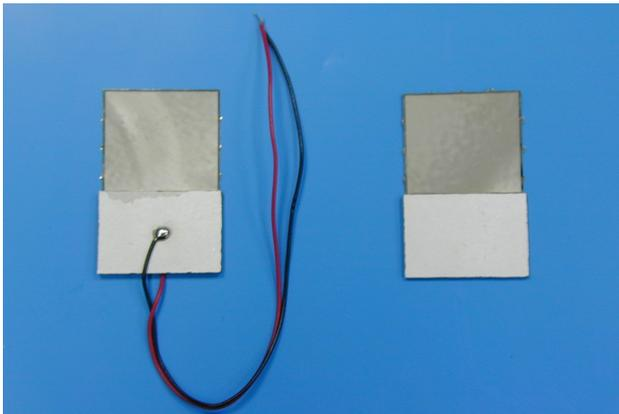
The ultrasonic vibration micro nozzle consists a piezoelectric ceramic and a metal foil, on which over thousands micro nozzles formed. Using the same principle as inkjet printer, this transducer atomizes water or liquids through a matrix of micro holes of around 7-10  $\mu\text{m}$ .
