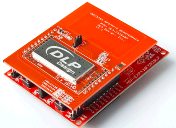
Figure 33. F5529 LaunchPad With DLP-7970ABP NFC BoosterPack
