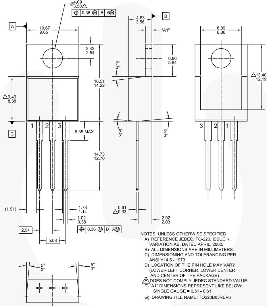
**Figure 5. TO-220, MOLDED, 3-LEAD, JEDEC VARIATION AB**
