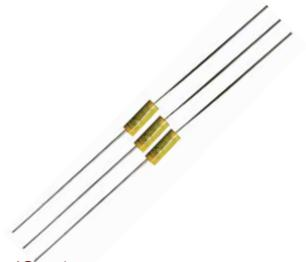
Type WMC axial-leaded polyester film/foil capacitors are ideal for automatic insertion in printed circuit boards. It is an ultraminiature version of Type WMF and the sections of these non-inductive capacitors are constructed with extended foil, polyster film, with tinned copper-clad steel leads.
